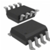
ADUM3123ARZ Analog Devices Inc. DGTL ISO 3KV GATE DRIVER 8SOIC
