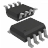
ADUM3123BRZ Analog Devices Inc. DGTL ISO 3KV GATE DRIVER 8SOIC
