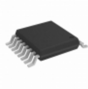
MAX4702EUE+ Maxim Integrated IC SWITCH QUAD SPDT 16TSSOP
