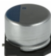
APXA160ARA331MJC0S United Chemi-Con CAP ALUM POLY 330UF 20% 16V SMD
