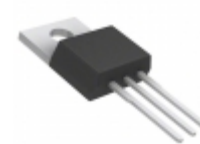
FCP11N65F Fairchild/ON Semiconductor MOSFET N-CH 650V 35A TO220
