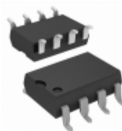
HCNW3120-300E Broadcom Limited OPTOISO 5KV GATE DRIVER 8DIP GW
