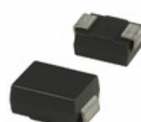
SMBJ78CA Fairchild/ON Semiconductor TVS DIODE 78VWM 126VC SMB
