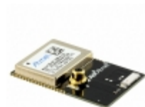
ATZB-RF-212B-0-CN Microchip Technology RF TXRX MODULE 802.15.4 CHIP ANT
