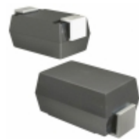
3SMAJ5918B-TP Micro Commercial Co DIODE ZENER 5.1V 3W DO214AC
