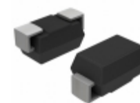
SMAJ7.5A Bourns Inc. TVS DIODE 7.5VWM 12.9VC DO214AC
