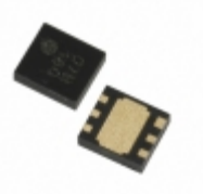
XC6123E522ER-G Torex Semiconductor Ltd IC WATCHDOG TIMER 6-USP
