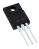
TSM60NB150CF C0G TSC (Taiwan Semiconductor) MOSFET N-CH 600V 24A ITO220S
