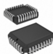
AT28HC256-70JU Microchip Technology IC EEPROM 256KBIT 70NS 32PLCC
