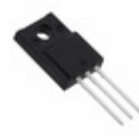
STFU6N65 STMicroelectronics N-CHANNEL 650 V, 1.2 OHM TYP., 4
