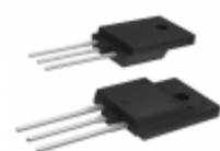
STFW20N65M5 STMicroelectronics MOSFET N-CH 650V 18A TO-3PF
