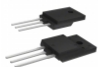
STFW12N120K5 STMicroelectronics MOSFET N-CH 1200V 12A TO-3PF
