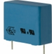
B32923C3105K EPCOS (TDK) CAP FILM 1UF 10% 305VAC RADIAL
