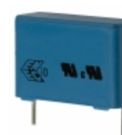
B32923A2474M EPCOS (TDK) CAP FILM 0.47UF 20% 305VAC RAD
