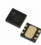
XC6121D428ER-G Torex Semiconductor Ltd IC WATCHDOG TIMER 6-USP
