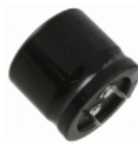
LGNW6271MELB30 Nichicon CAP ALUM 270UF 20% 420V SNAP
