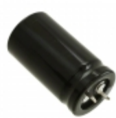
LGNW6181MELZ40 Nichicon CAP ALUM 180UF 20% 420V SNAP
