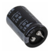
LGNW6271MELA40 Nichicon CAP ALUM 270UF 20% 420V SNAP
