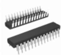
PIC18F24Q10-I/SP Micrel / Microchip Technology 16KB FLASH, 1KB RAM, 256B EEPROM
