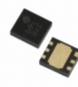
XC6121D532ER-G Torex Semiconductor Ltd IC WATCHDOG TIMER 6-USP
