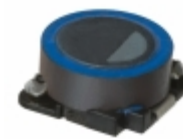
SLF7032T-681MR16-2PF TDK Corporation FIXED IND 680UH 160MA 3.78 OHM
