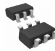
NCP308SN250T1G ON Semiconductor IC SUPERVISOR 2.5V TSOP6
