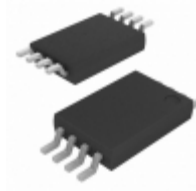
AT93C56B-XHM-B Microchip Technology IC EEPROM 2KBIT 2MHZ 8TSSOP
