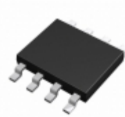
BR24G08FVM-3AGTTR Rohm Semiconductor IC EEPROM 8KBIT 1MHZ 8MSOP
