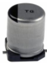
EEE-TG1V471M Panasonic Electronic Components CAP ALUM 470UF 20% 35V SMD
