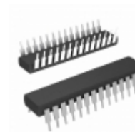
PIC32MX250F128B-50I/SP Microchip Technology IC MCU 32BIT 128KB FLASH 28SDIP
