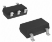
AN80L30RMS Panasonic Electronic Components IC REG LDO 3V 0.15A MINI5D
