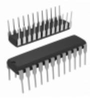
ADM238LANZ Analog Devices Inc. IC TXRX RS-232 4:4 5V LP 24DIP
