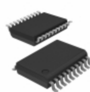
PIC16C558-04/SS Microchip Technology IC MCU 8BIT 3.5KB OTP 20SSOP
