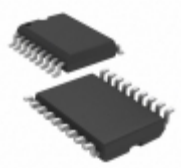
PIC16C620-20I/SO Microchip Technology IC MCU 8BIT 896B OTP 18SOIC
