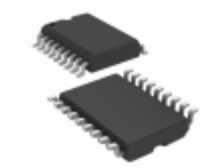
PIC16C620-20E/SO Microchip Technology IC MCU 8BIT 896B OTP 18SOIC
