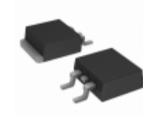
T810H-6G STMicroelectronics TRIAC SENS GATE 600V 8A D2PAK
