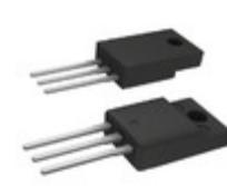
T810T-8FP STMicroelectronics TRIAC SENS GATE 800V 8A TO-220FP
