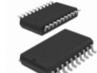
MM74HCT245SJ Fairchild/ON Semiconductor IC TRANSCVR TRI-ST 8BIT 20SOP
