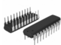
MM74HCT245N Fairchild/ON Semiconductor IC TRANSCVR TRI-ST 8BIT 20DIP
