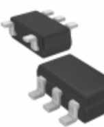
XC6121D617MR-G Torex Semiconductor Ltd IC WATCHDOG TIMER SOT-25
