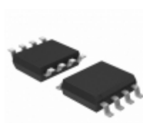
TC4429EOA Microchip Technology IC MOSFET DRIVER 6A INV 8SOIC
