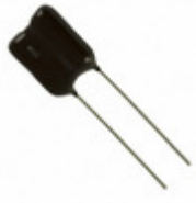
CD30FD362FO3 Cornell Dubilier Electronics (CDE) CAP MICA 3600PF 1% 500V RADIAL
