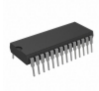
AT28BV256-20PI Microchip Technology IC EEPROM 256KBIT 200NS 28DIP
