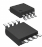
PIC12F510T-I/MS Microchip Technology IC MCU 8BIT 1.5KB FLASH 8MSOP
