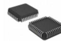
TS87C54X2-LCB Microchip Technology IC MCU 8BIT 16KB OTP 44PLCC
