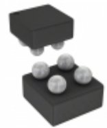
M24C08-FCT6TP/T STMicroelectronics IC EEPROM 8KBIT 400KHZ 4WLCSP
