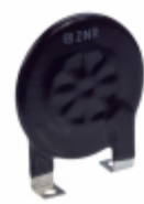
ERZ-C40CK751W Panasonic Electronic Components VARISTOR 750V 30A DISC 40MM
