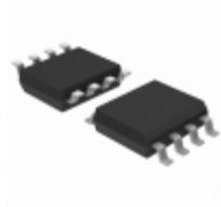
AT45DB041E-SHNHC-T Adesto Technologies IC FLASH 4MBIT 85MHZ 8SOIC
