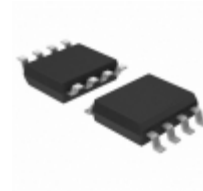
AT45DB041E-SSHNHA-T Adesto Technologies IC FLASH 4MBIT 85MHZ 8SOIC
