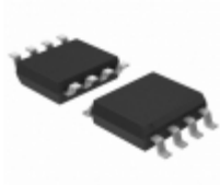
PIC12HV609-E/SN Microchip Technology IC MCU 8BIT 1.75KB FLASH 8SOIC
