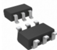
LTC3560IS6#TRMPBF Linear Technology IC REG BUCK ADJ 0.8A SYNC TSOT23
