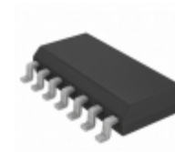
PIC16LF15323T-I/SL Micrel / Microchip Technology IC MCU 8BIT 3.5KB FLASH 14SOIC
