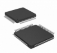
PIC24FJ256GB206-I/PT Microchip Technology IC MCU 16BIT 256KB FLASH 64TQFP
