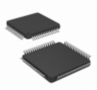
PIC24FJ256GB106T-I/PT Microchip Technology IC MCU 16BIT 256KB FLASH 64TQFP
