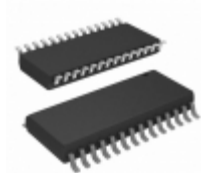
AT45D081-RI Microchip Technology IC FLASH 8MBIT 15MHZ 28SOIC
