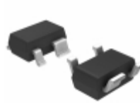
S-1000C30-N4T1G SII Semiconductor Corporation IC VOLT DETECTOR 30V SC-82AB
