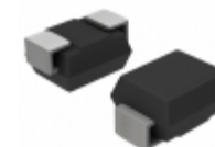
1SMB5944BT3 ON Semiconductor DIODE ZENER 62V 3W SMB
