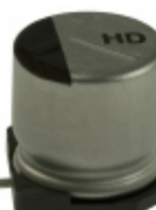
EEV-HD1V101P Panasonic Electronic Components CAP ALUM 100UF 20% 35V SMD
