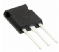
APT36GA60B Microsemi Corporation IGBT 600V 65A 290W TO-247
