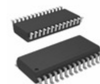
CY7C64013A-SXC Cypress Semiconductor Corp IC MCU 8K FULL SPEED USB 28SOIC
