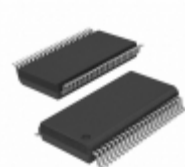
CY7C63923-PVXC Cypress Semiconductor Corp IC USB PERIPHERAL CTRLR 48SSOP
