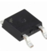
FGD4536TM Fairchild/ON Semiconductor IGBT 360V 125W DPAK
